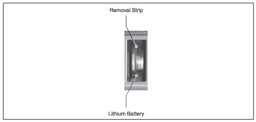
Figure 4: CP570 removal strip should be pulled to the right
