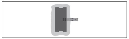
Figure 2: Removing the CP570 cover for the lithium battery
