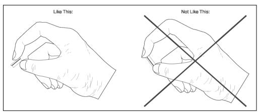
Figure 3: Correct grip for the CP570 battery
