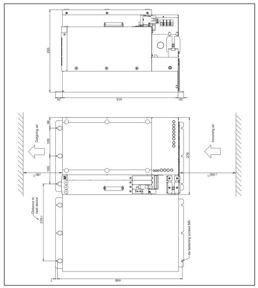
Figure 11: Dimensional diagram and installation dimensions for ACOPOS 1640
