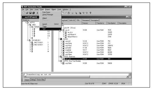
Figure 63: Command to open the test window
