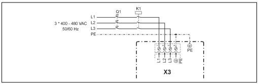
Figure 17: Circuit diagram for ACOPOS X3, individual power mains connection
