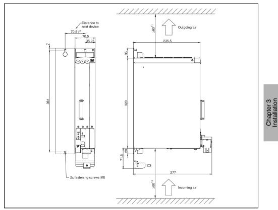
Figure 10: Dimensional diagram and installation dimensions for ACOPOS 1022, 1045, 1090
