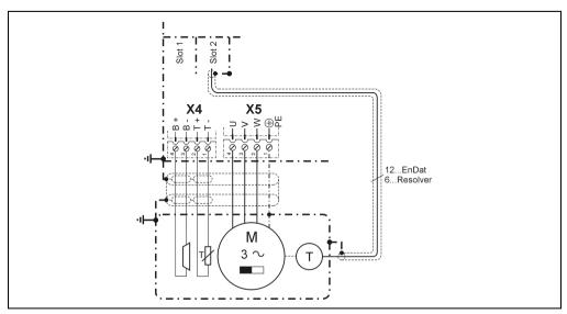
Figure 20: ACOPOS X4/X5 circuit diagram, motor connection
