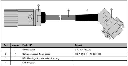
Table 71: Resolver cable construction
