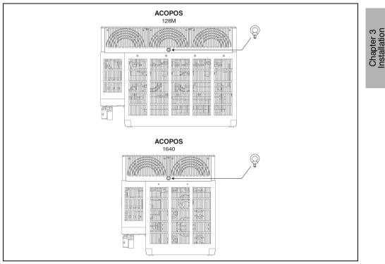
Figure 9: Attaching the ring screws contained in the delivery to ACOPOS 1640 and 128M drives
