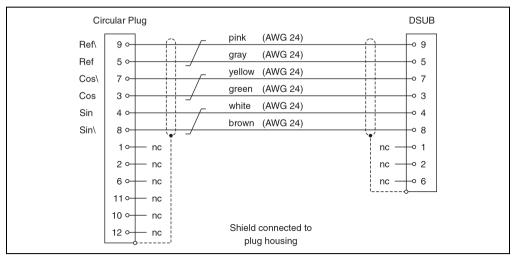
Figure 30: Cable schematic for resolver cables
