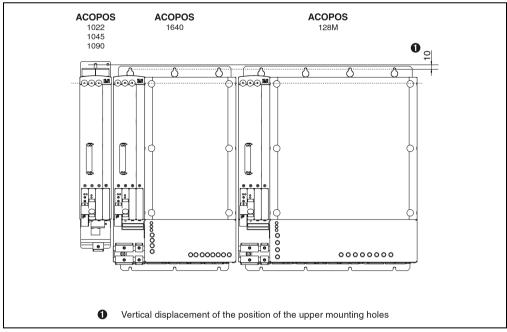
Figure 14: Installing various ACOPOS series devices directly next to each other
