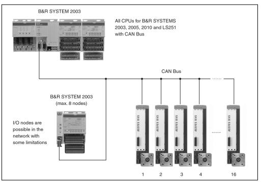
Figure 7: CAN Configuration 1
