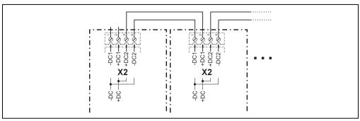
Figure 19: ACOPOS X2 circuit diagram, DC bus connections
