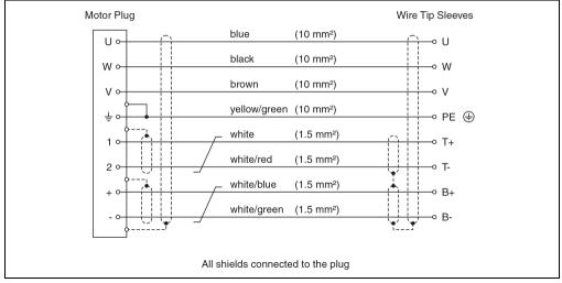
Figure 28: Cable schematic for motor cables 8CMxxx.12-5
