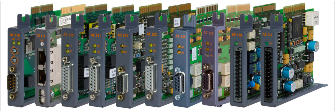
Figure 2: Plug-in modules allow optimized, application-specific configuration of ACOPOS servo drives
