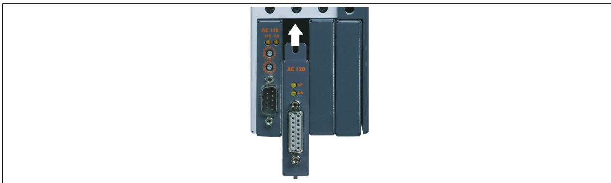
Figure 60: Installing ACOPOS plug-in modules
