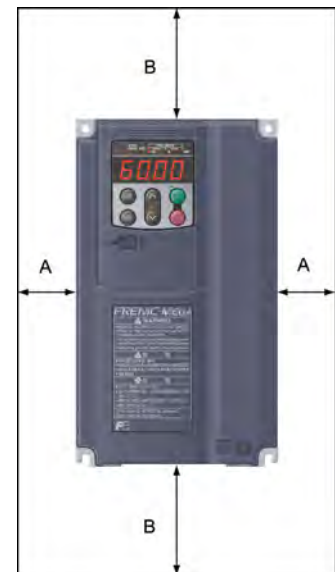
Figure 2.1 Mounting Direction and Required Clearances
